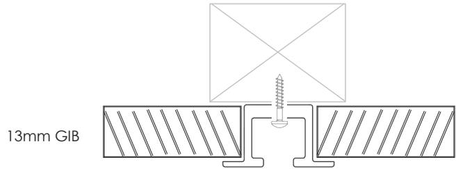
Flush Fit Track is a track recessed into the ceiling. The track sits inside the ceiling lining and requires no brackets for installation. Flush Fit track is 13mm high which is the standard thickness of ceiling lining sheet used in New Zealand (GIB) and Australia (Gyprock).
